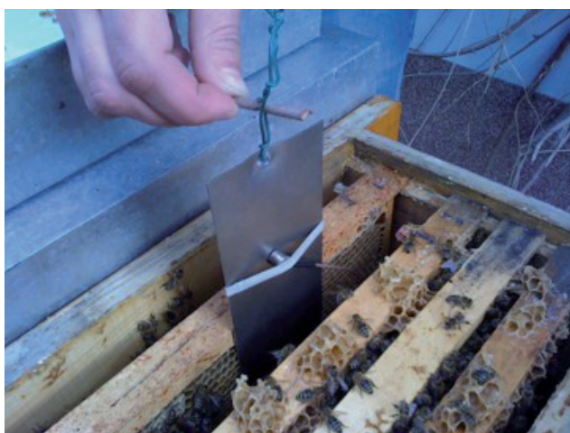
2: Slot01-02 sensors on the sheet metal plate in the hive interior. Photo by authors.
